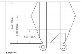
Standard flights are available in 2", 3" and 4" heights. Standard Sideplates are available in standard 1", 2", and 3" heights. flight indent is 1" or greater from outside edge of belt.
