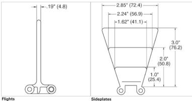
Standard flights are available in 1", 2", and 3" heights. Standard flight indent is 1" or greater from outside edge of belt.
