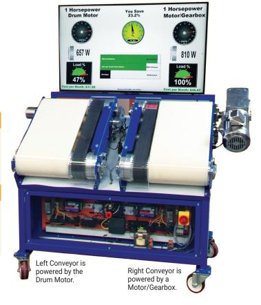
The tests revealed that the conveyor powered by the Van der Graaf drum motor saves 23% energy when compared to the conventional conveyor drive. The drum motor, while producing the same torque as the motor/ gearbox, is operating at a fraction of its full capacity, extending the life span of the drive as well as reducing maintenance.
