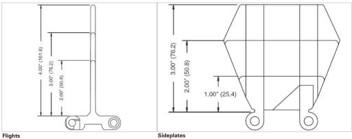
Standard flights are available in 2°, 3° and 4° heights. Standard Sideplates are available in standard 1°, 2°, and 3° heights. flight indent is 1° or greater from outside edge of belt.
