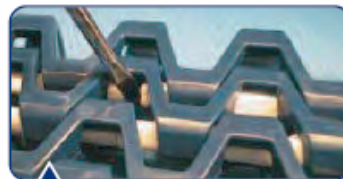
Use flat blade screwdriver to pry out the rods.
