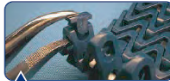
Use nose pliers to put plug into final position.
