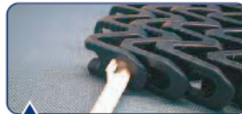
Rotate pins approx. 45° and slide pin into the belt (one from each side and thick end first).
