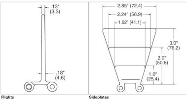
Flights Standard flights are available in 1", 2", and 3" heights. Standard flight indent is 1" or greater from outside edge of belt.
