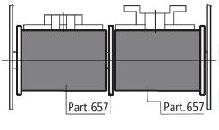
Double roller with rubber surface 2.36" dia.
